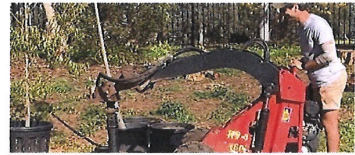
Holes for the new trees were made using an auger drill.
